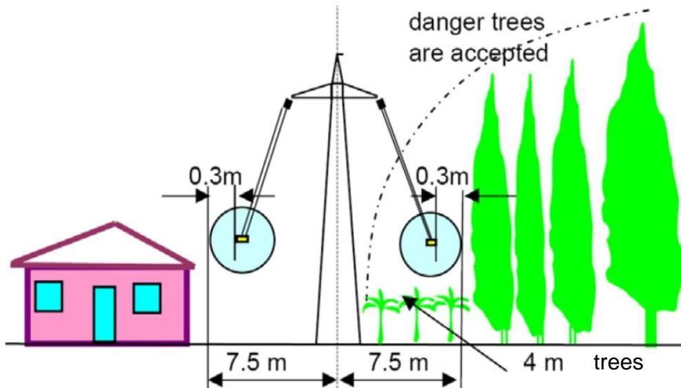
**Figure 6.2 – Typical Electrode line Corridor clearance considerations**
