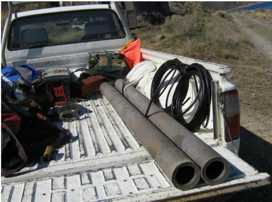
**Figure 5.41 - New electrode elements (high silicon-chromium iron)**
