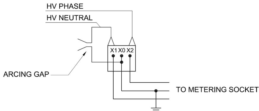
Figure 7.2 - Isolation of Distribution System Multi-grounded Neutral at Grounding Site
