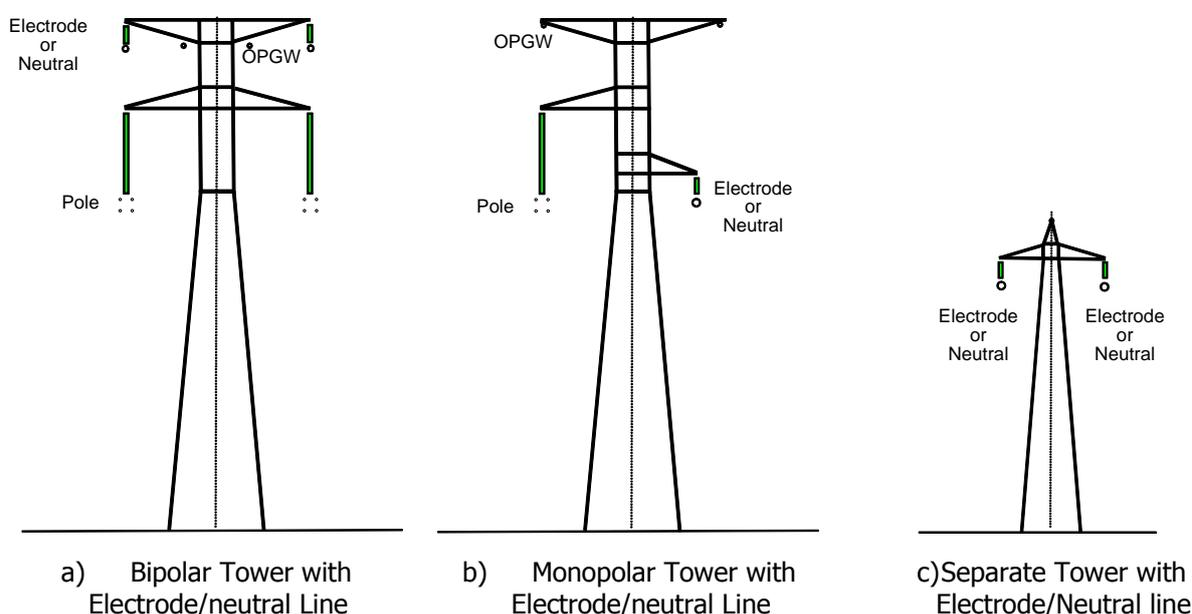
**Figure 6.1 - Conceptual electrode line configurations**
