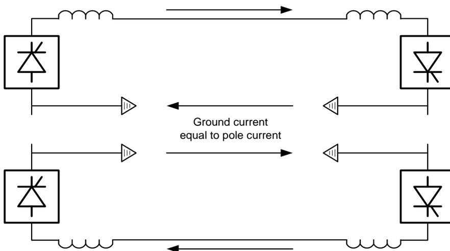
**Figure 1.1 - Monopole Configurations with Electrodes**
