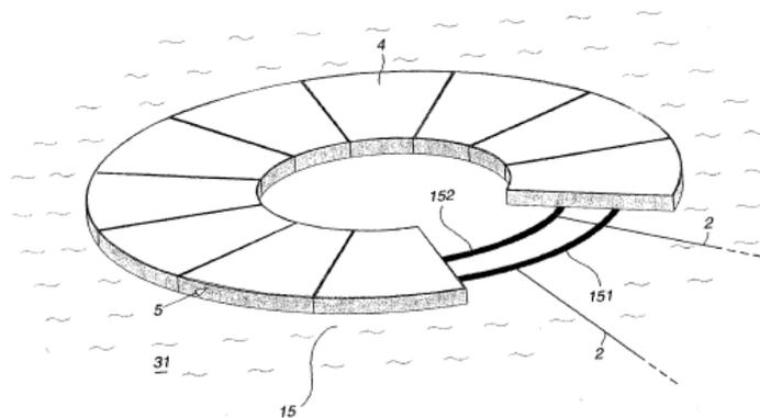
**Figure 5.23 - Sea Electrode with Two Concentric Rings as Electrode Body and Ballast [60]**
