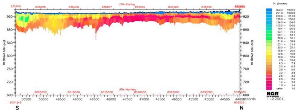
Figure 3.9 - Vertical section based on one of the flight lines from the Caprivi helicopter-borne survey of Figure 3.8
