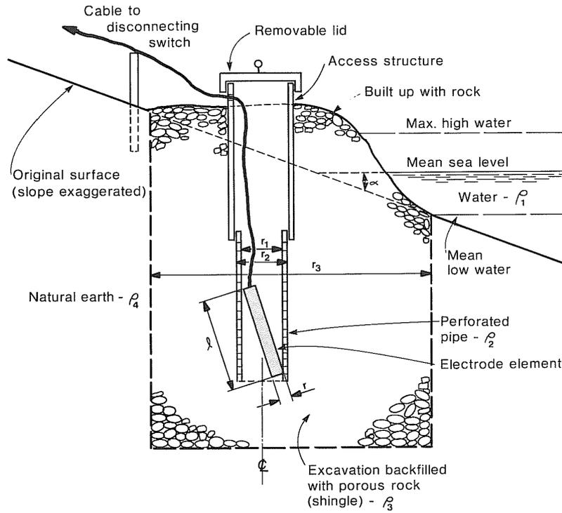
Figure 2.14 - Profile View of Beach Electrode in Shallow Well [1]
