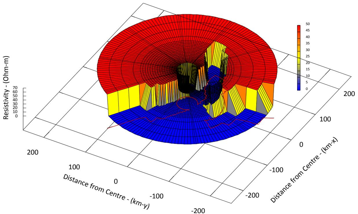
**Figure 5.8 - Example of A Top Layer Resistivity as Modeled In Area Within 250km Of The Electrode**
