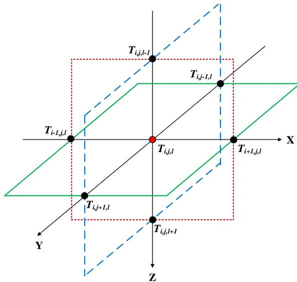
Figure 5.12 – Internal Node Located in XYZ planes
