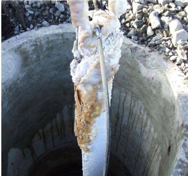
**Figure 5.39 - Electrode element with deposit build-up, typical for cathodic Operation**
