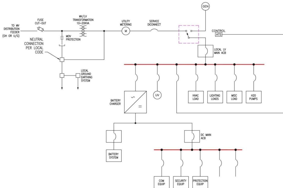
Figure 7.1 - Typical Single line Diagram
