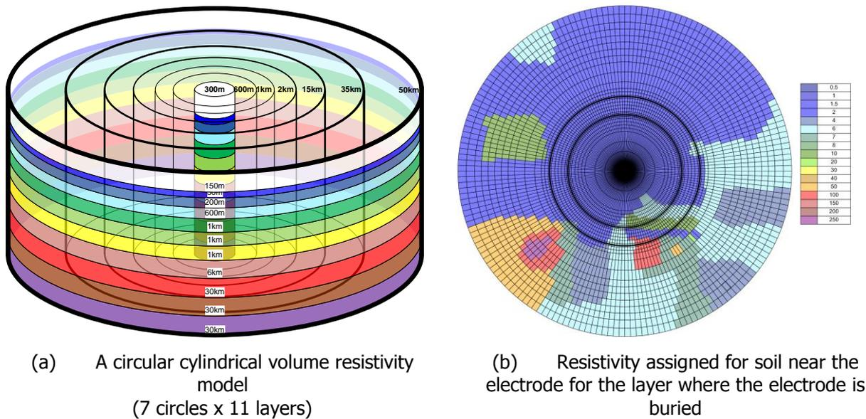
**Figure 5.7 – Example of circular cylindrical volume resistivity model**
