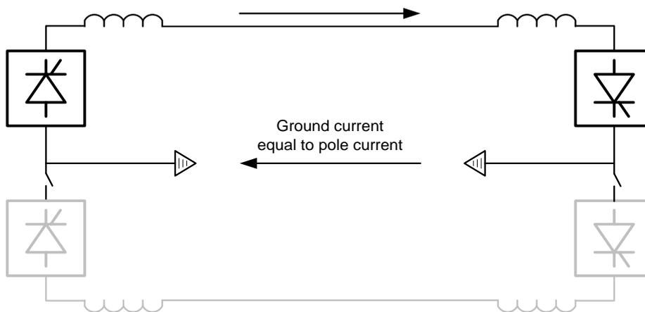
**Figure 1.3 - Bipolar Configuration Operated as A monopole with Electrodes**
