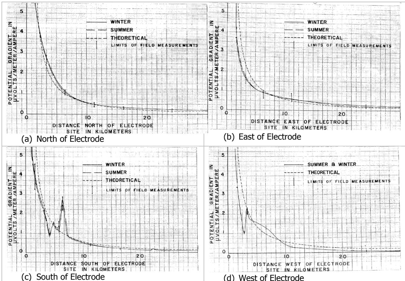
**Figure 8.6 – Potential Gradient Measurement (Manitoba Nelson River HVDC Electrode) [79]**
