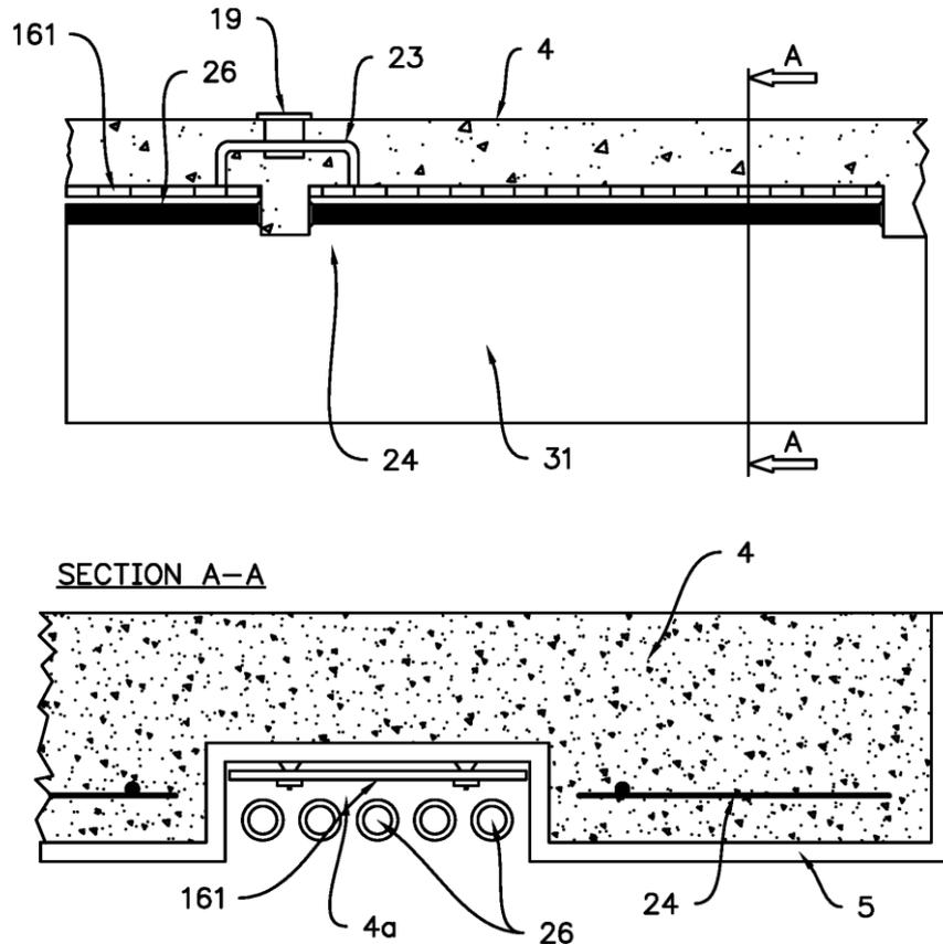
**Figure 5.28 - Side View of a Part of an Electrode with Flat sub-electrode Elements Located within Cavities in a Concrete Plate and A section View along the Line A-A [60]**
