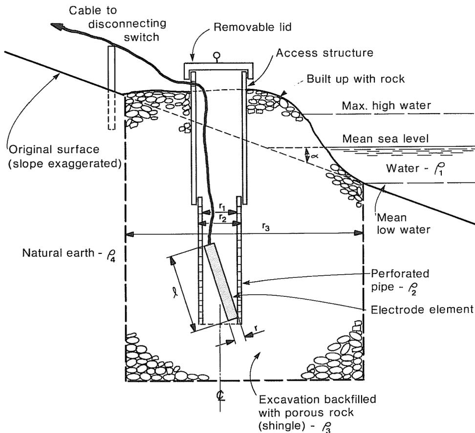
**Figure 5.37 - Cross-section of typical beach electrode arrangement [1]**
