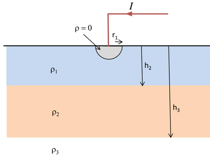
**Figure 3.5 – Electrode model consisting of horizontal layers**
