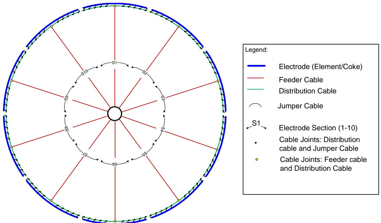
**Figure 0.2 - Conceptual diagram showing a ring electrode connection**
