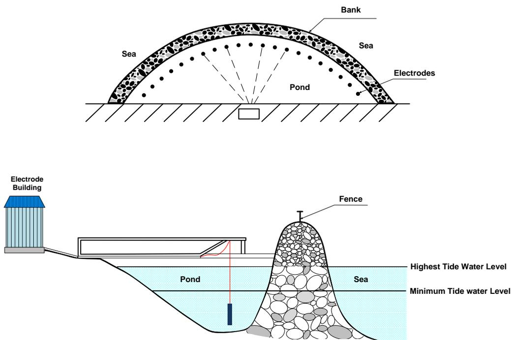
**Figure 5.31 - Shoreline Pond Electrode-Suspended Electrode Element**
