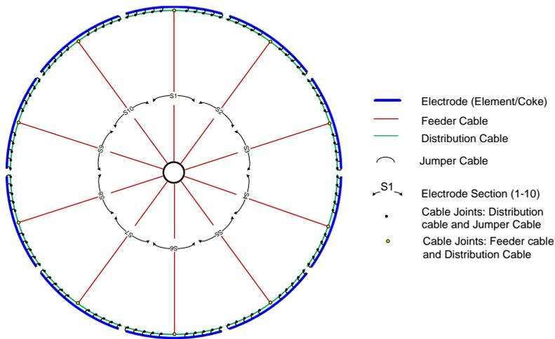
**Figure 2.3 - Ring Electrode Arrangement**
