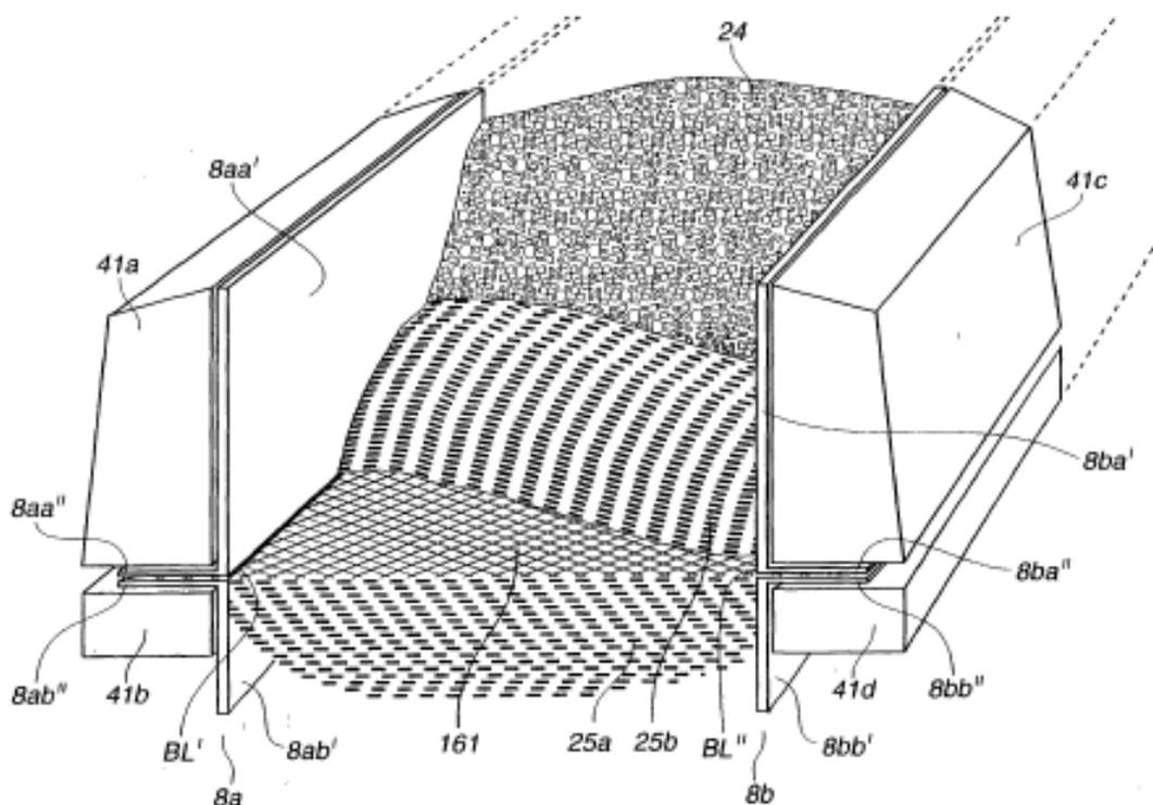
**Figure 5.30 - A Sub-electrode Element Embedded in a Backfill [60]**
