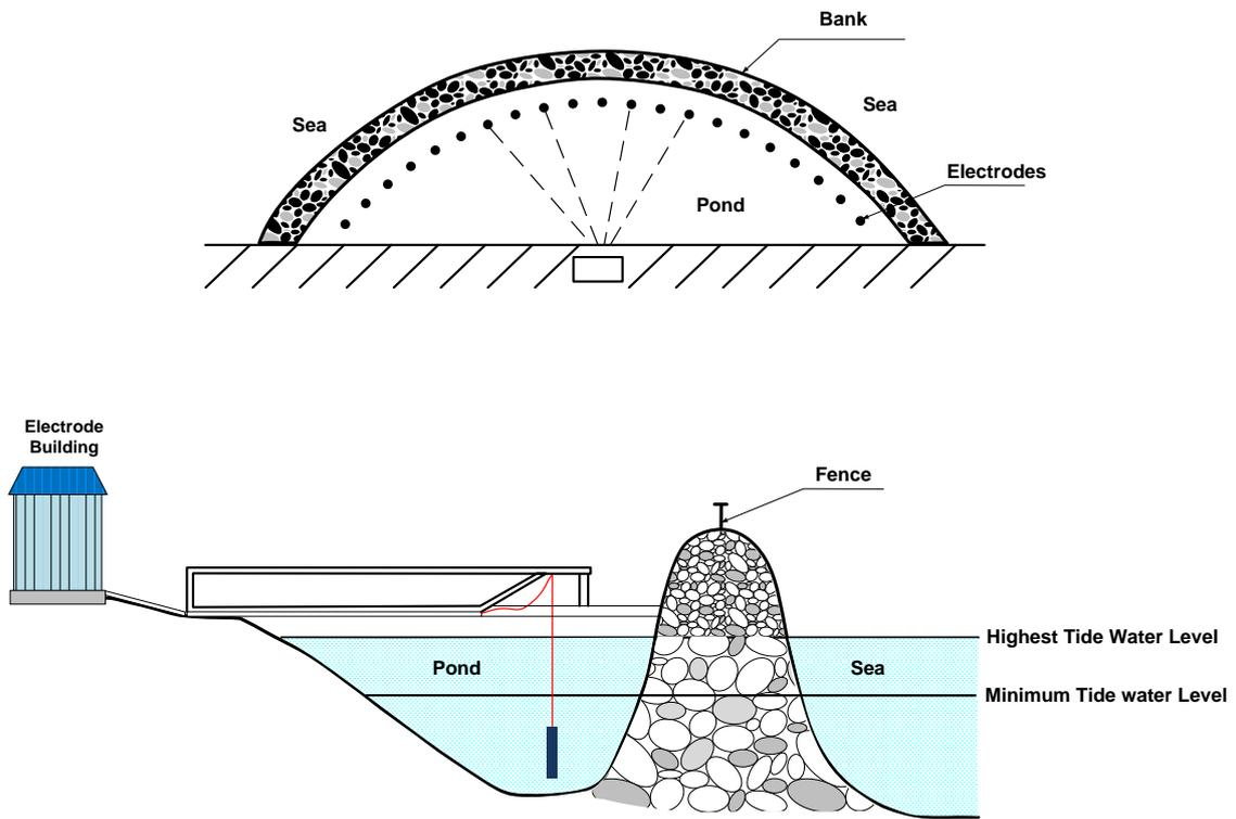
**Figure 2.16 - Conceptual Plan and Profile Views of a Pond Electrode**
