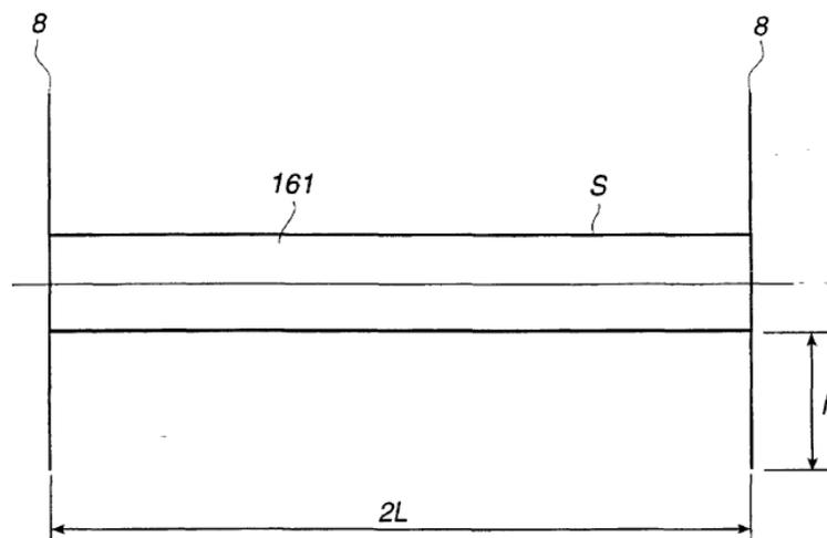
**Figure 5.25 - Cylinder Shaped Sub-electrode Element Provided with Non-conducting Barriers [60]**
