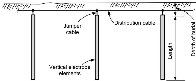
**Figure 2.5 - Vertical Electrode (placed in a line, ring, or arbitrary arrangement)**
