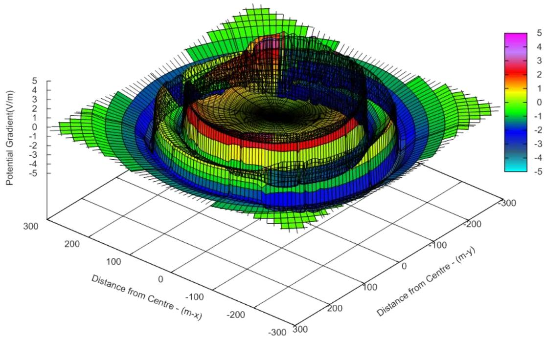
**Figure 5.10 - Example of A Local Calculated Potential Gradient of A Shallow Double Ring Electrode**
