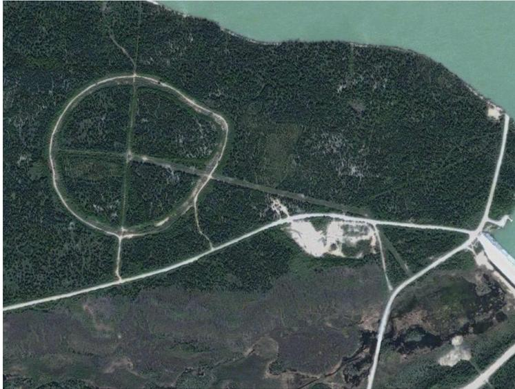
**Figure 2.4 - Land Electrode (Manitoba Bipole 1 – Radisson)**
