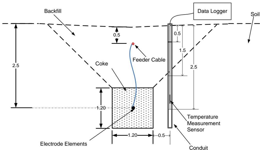
**Figure 8.1 - Soil Temperature Measurement Diagram**
