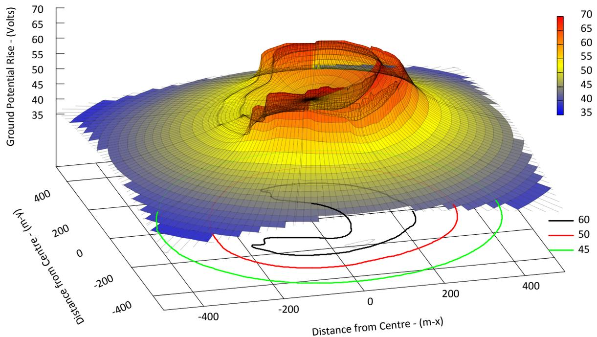
**Figure 5.9 - Example of Calculated Ground Potential Rise near A Shallow Double Ring Electrode With A Portion of The Electrode Out of Service**
