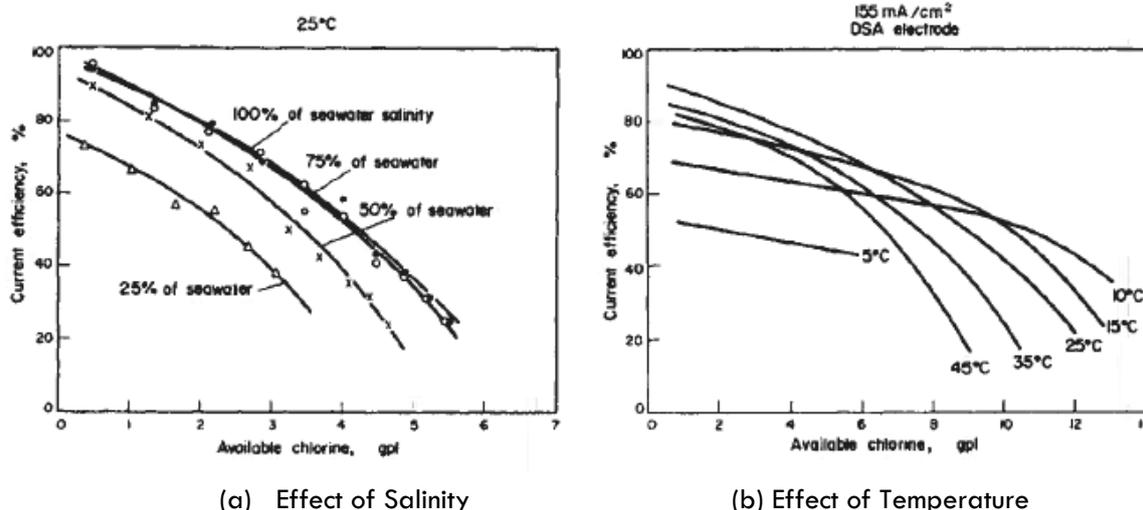
Figure 5.20 - Current Efficiency vs Available Chlorine Concentration using DSA Anodes [59]
