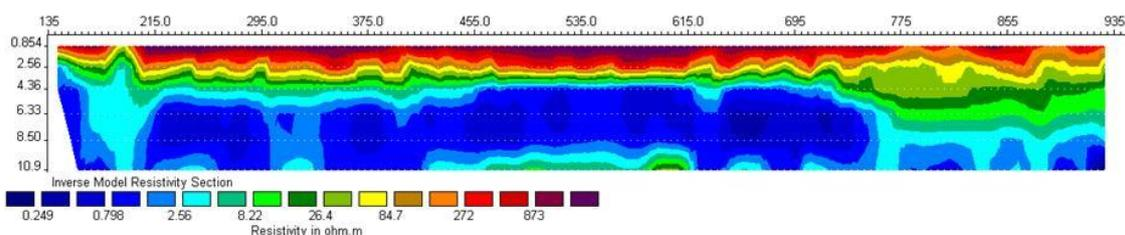
**Figure 3.12 - ground SHALLOW resistivity profile (courtesy of NamPower)**
