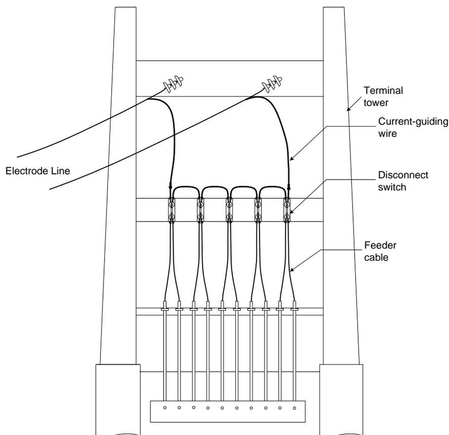
**Figure 0.1 - Conceptual diagram showing the electrode current guiding system**
