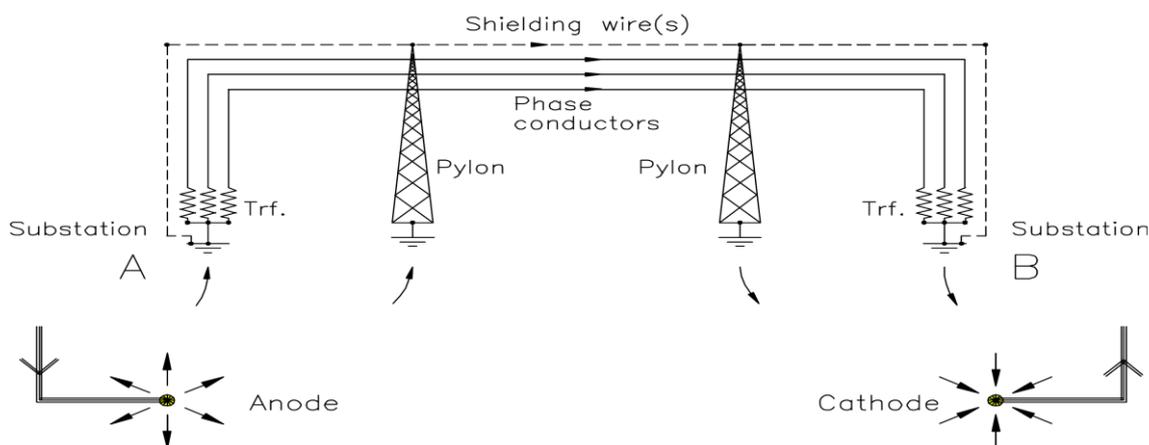
**Figure 4.1 – Overview of ac connection exposed to a Field from two electrode stations**
