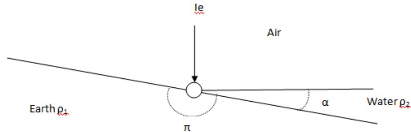
**Figure 5.35 - Shoreline Pond Electrode Simplified Model**
