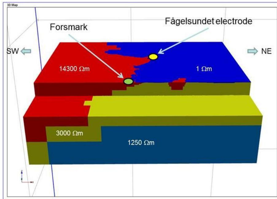
**Figure 3.10 - Regional resistivity model around the Fågelsundet electrode based on open-file data [12]**
