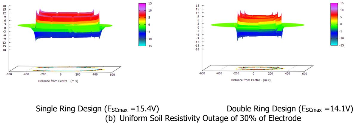
**Figure 5.17 – Simulated Potential gradient**
