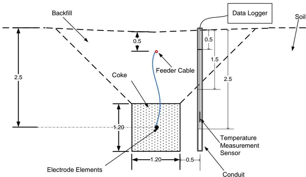
**Figure 8.1 - Soil Temperature Measurement Diagram**
