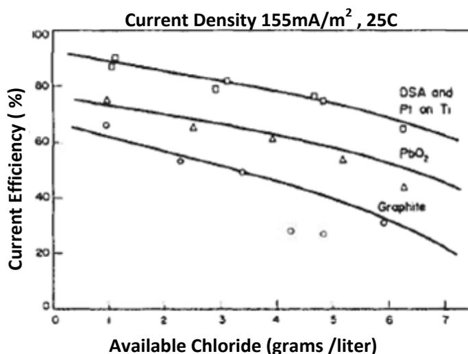
**Figure 5.19 - Current Efficiency vs. Available Chlorine Concentration in Seawater for Different Electrode Materials [59]**
