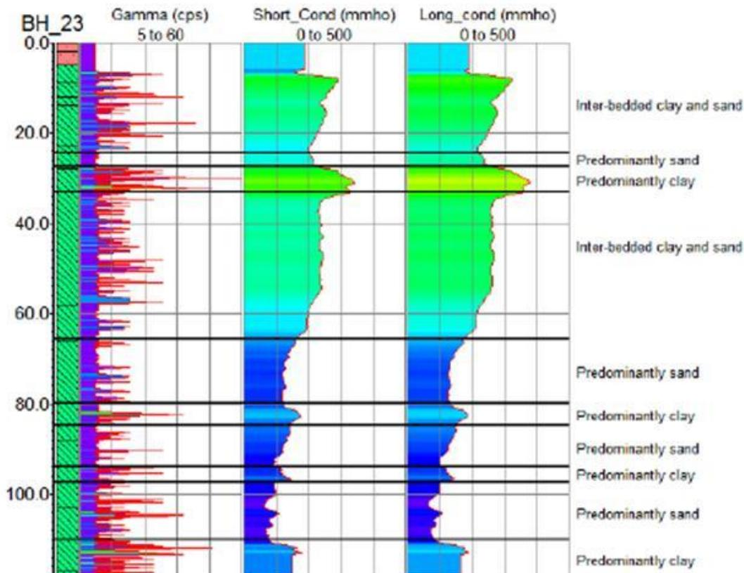
**Figure 3.14 – Results from down-hole electric conductivity and gamma radiation logging from a test hole at the Zambezi electrode site of the Caprivi Link**
