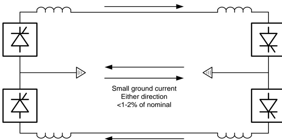
**Figure 1.2 - Bipolar Configuration with Electrodes**
