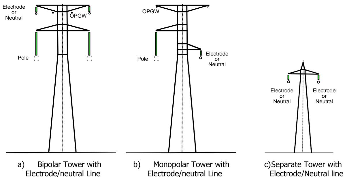
**Figure 6.1 - Conceptual electrode line configurations**
