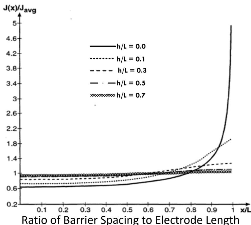
**Figure 5.24 - The effect of Non-conducting Barriers according to Figure 5.25 on the Current Distribution Along a Cylinder-shaped Sub-electrode Element [60]**
