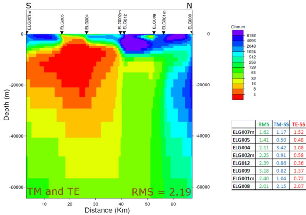
Figure 3.6 - Typical Resistivity Profile Provided by magnetotelluric survey
