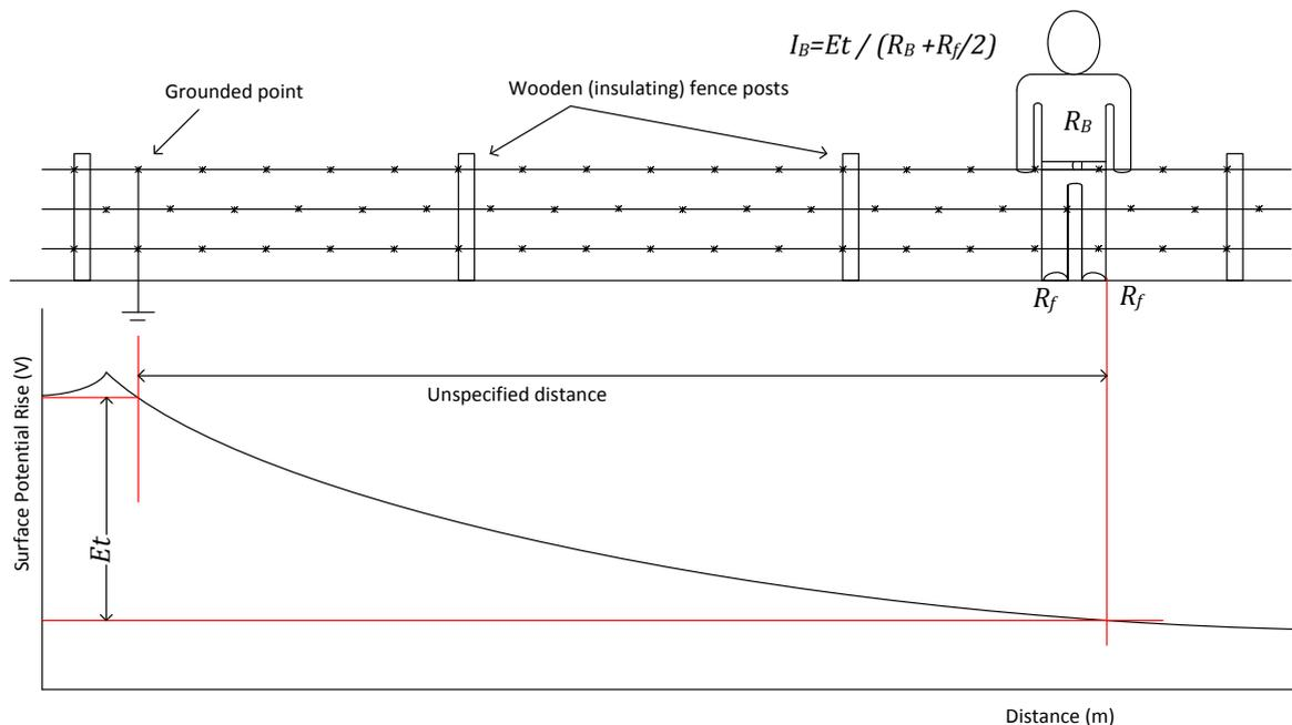
**Figure 5.4 – Conceptual Illustration of Transferred Potential**
