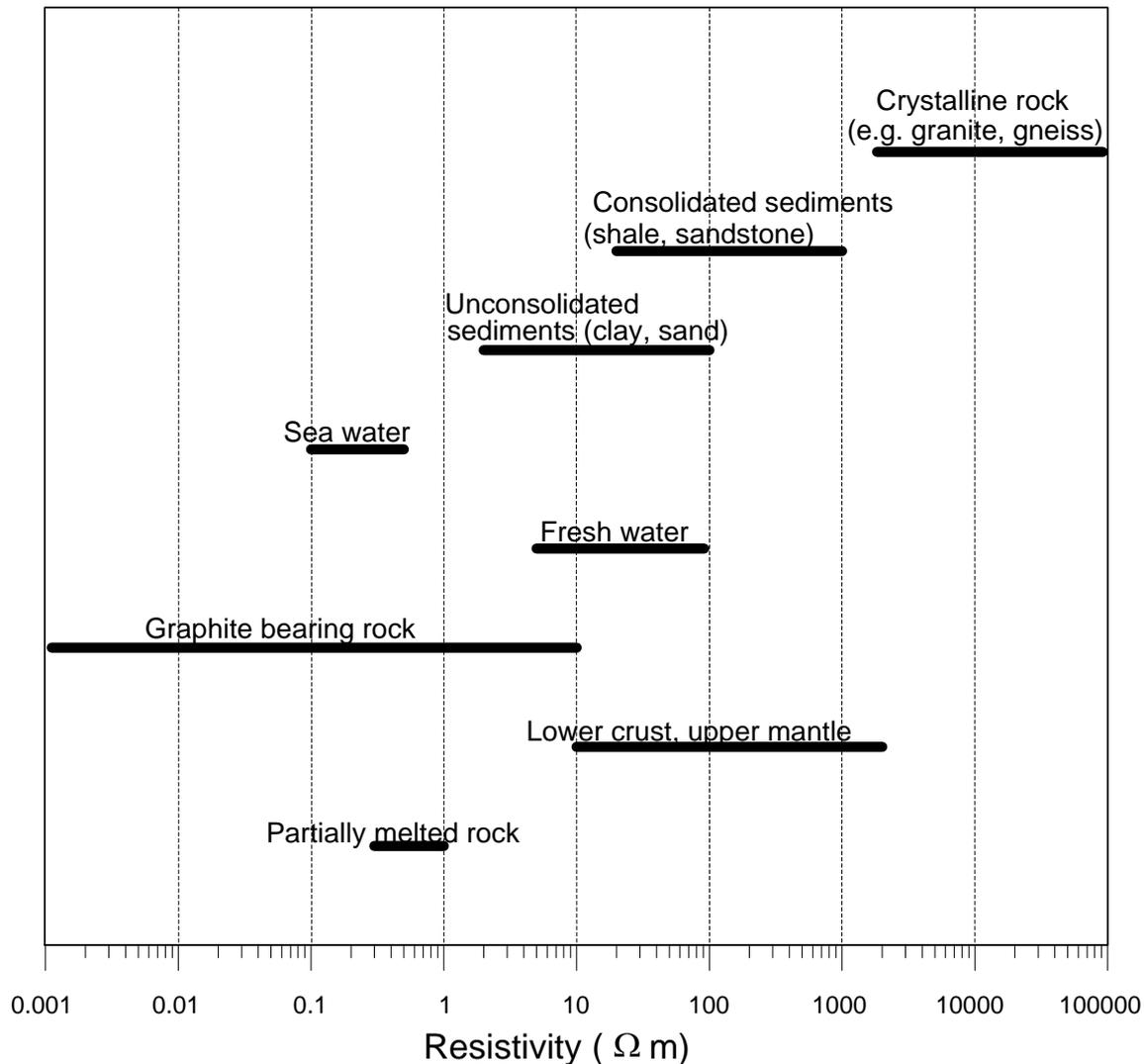
**Figure 3.3 - Approximate resistivity ranges for different types of geological Formations**
