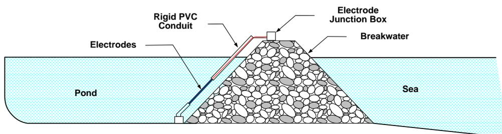
**Figure 5.32 - Shoreline Pond Electrode-Elements on Inside Face of Breakwater**
