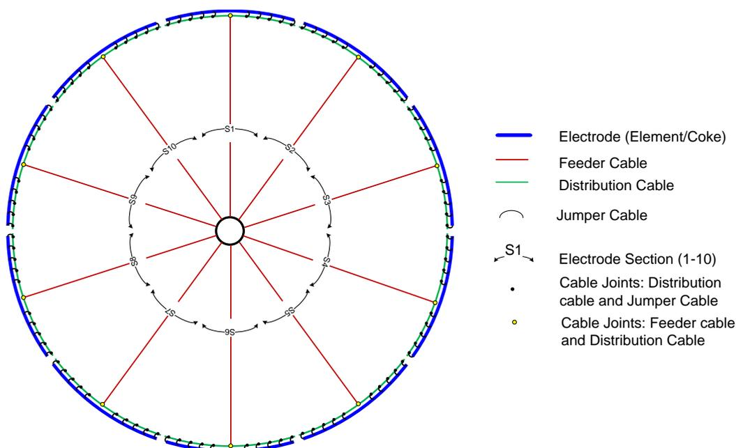
**Figure 5.15 - Single Shallow Ring Electrode Arrangement with Ten Sub-electrodes**
