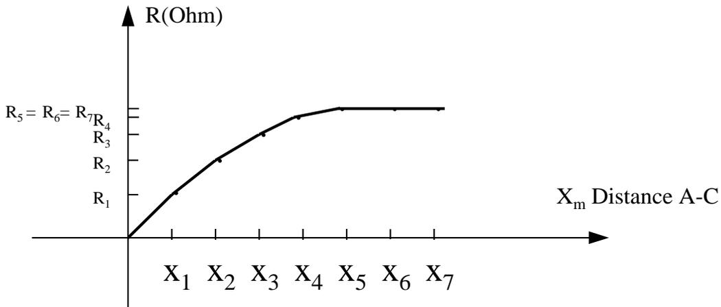
**Figure 8.3 - Impedance as a function of distance**
