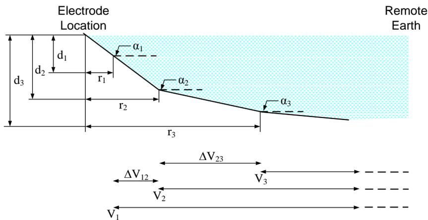
**Figure 5.36 - Model Representation with Varying Sea bed Slopes**
