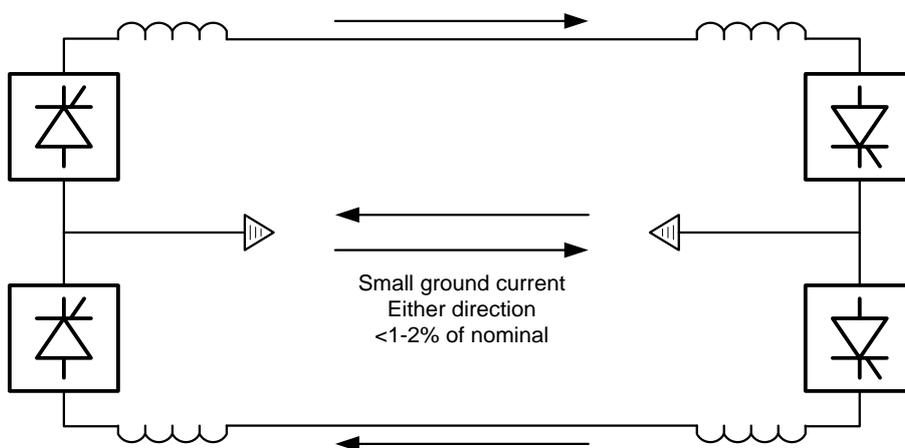
**Figure 1.2 - Bipolar Configuration with Electrodes**
