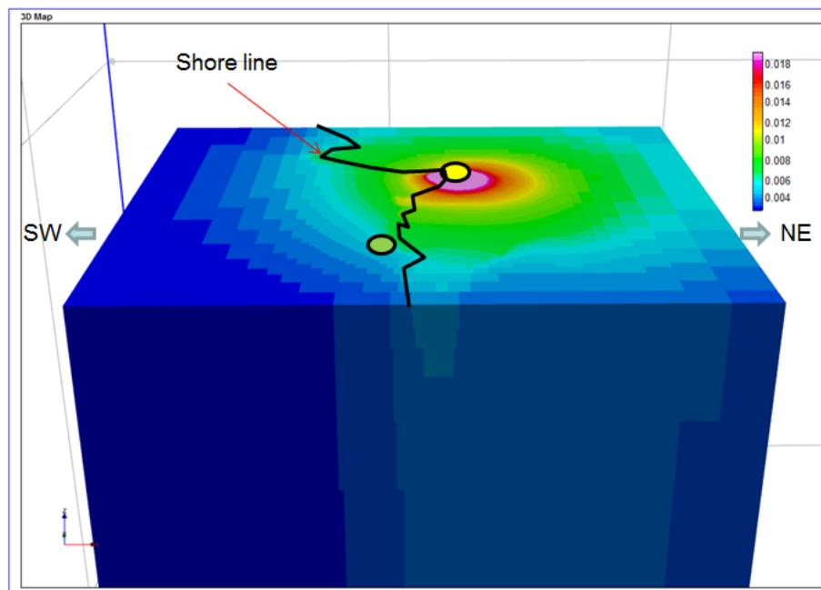
**Figure 3.11 - Calculated potential RISE due to current injection at Forsmark (Figure 3.10) into the resistivity model [12]**
