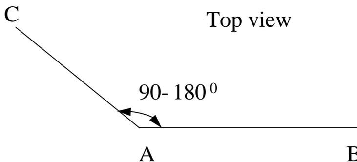
**Figure 8.4 - Angle between current line and potential conductor**
