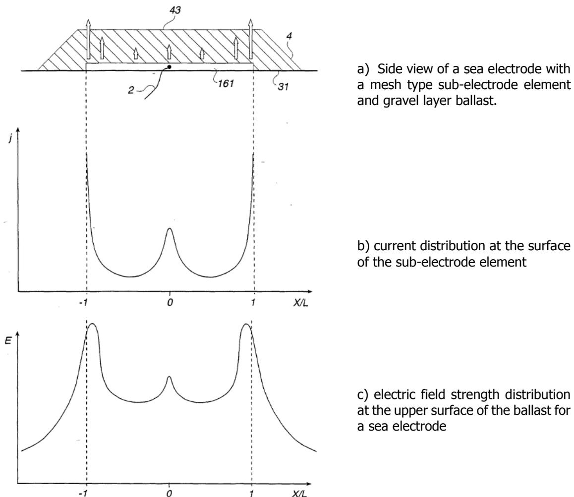
Figure 5.22 – Possible Configuration of Sea Electrode Mesh Covered with Gravel Ballast [60]
