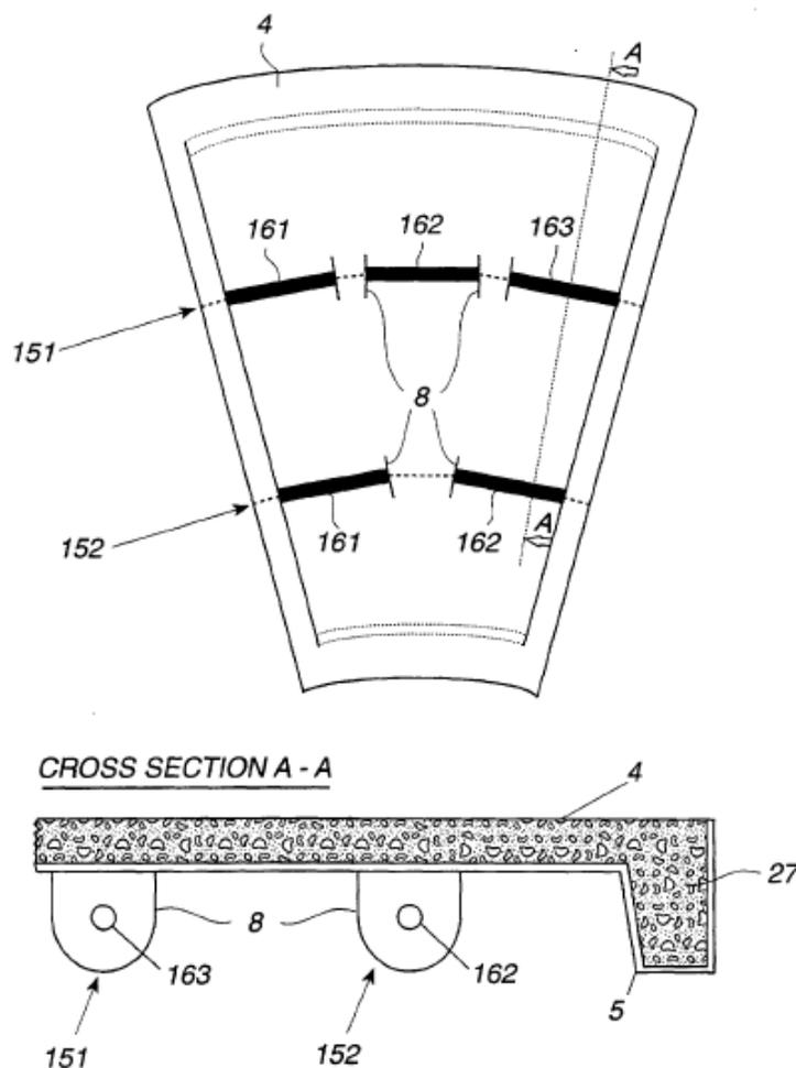
**Figure 5.29 - Section Of An Electrode, Seen from Below, With A Ballast in the Form of Concrete Plate with Coated Side Walls and A Section along The Line A-A [60]**
