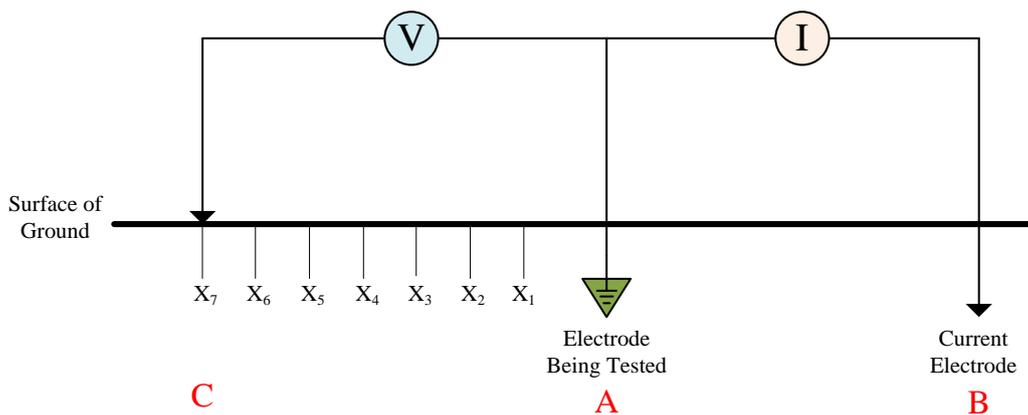
**Figure 8.2 - Measurement of resistance to remote earth**
