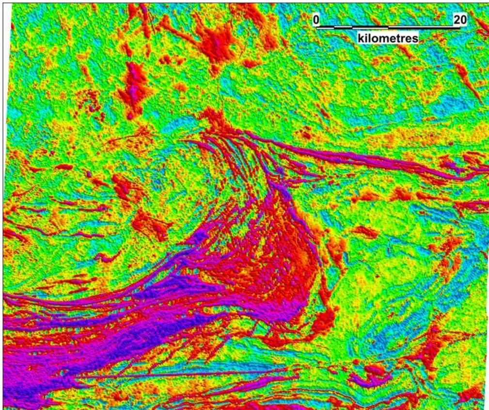
Figure 3.7 - Airborne electromagnetic measurements in Finland that highlight low-resistivity graphite bearing structures (red-purple) in the ground [9]
