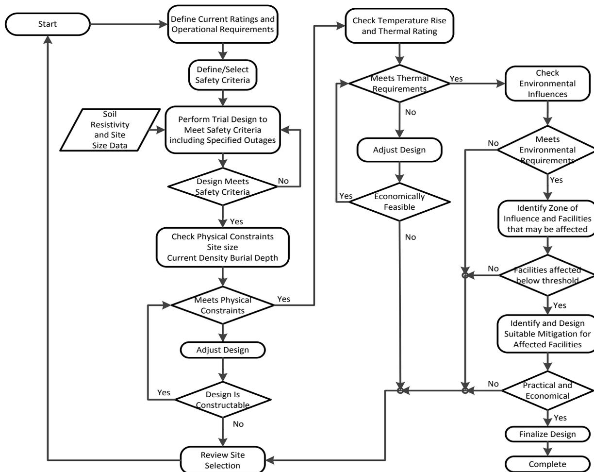
**Figure 5.1 – Conceptual flowchart of Electrode design Process**
