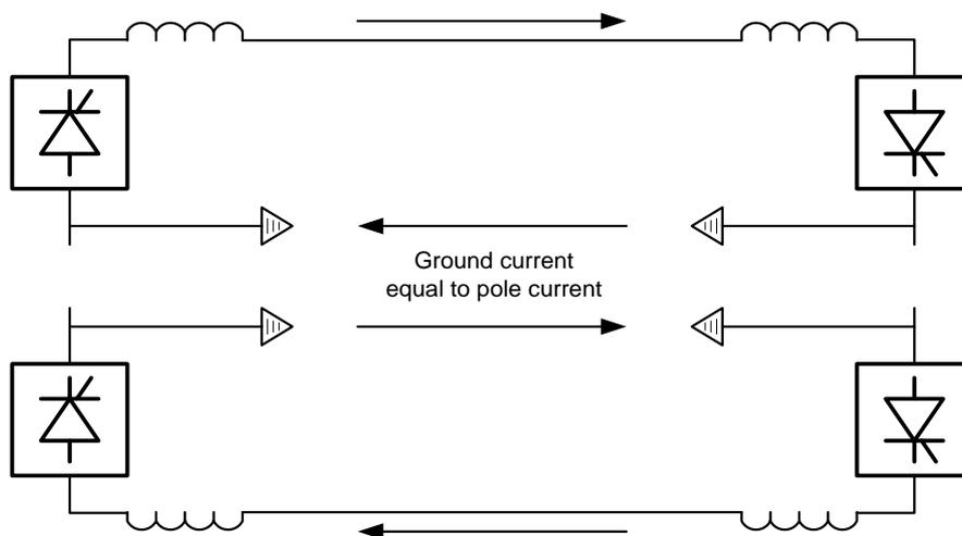
**Figure 1.1 - Monopole Configurations with Electrodes**
