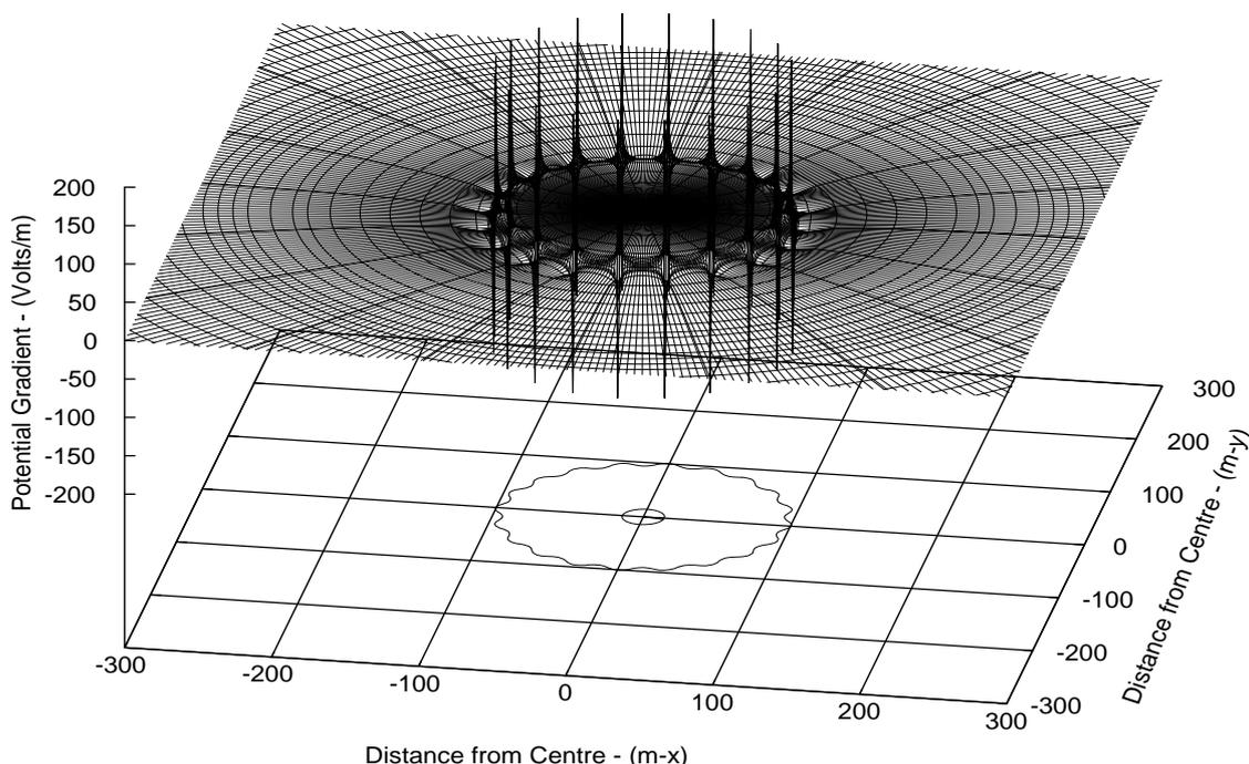
**Figure 5.11- Example of Calculated Potential Gradients from A Ring of Deep Well Electrodes**
