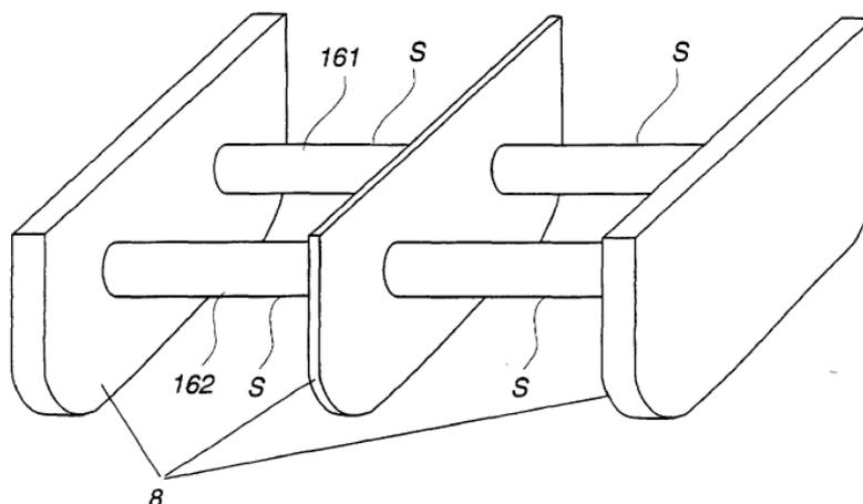
**Figure 5.26 - A Pair of Cylinder-shaped Sub-electrode Elements with Non-conducting Barriers, also Serving as Mechanical Supports [60]**
