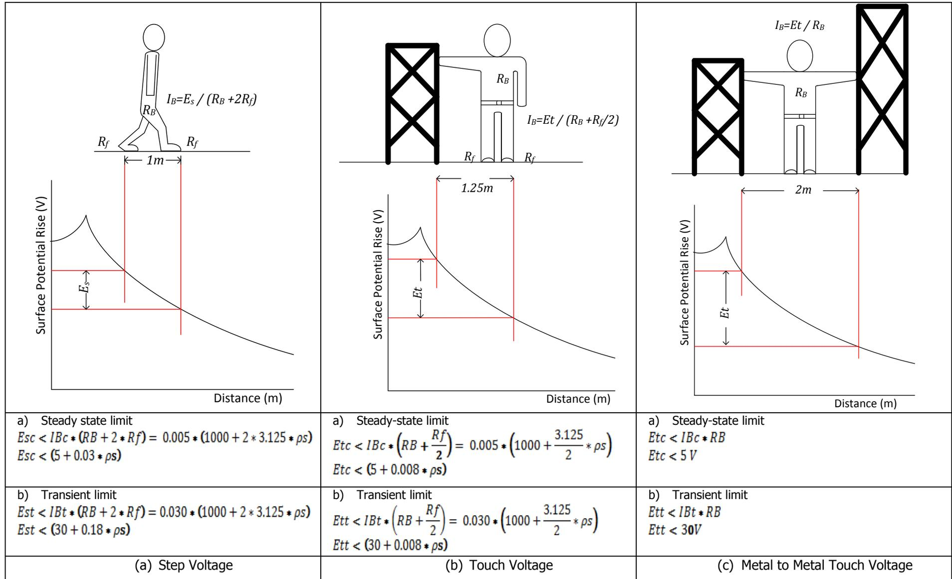
Figure 5.3 – Conceptual illustration of step voltage, touch Voltage and metal to metal touch voltage and corresponding Safety criterion
