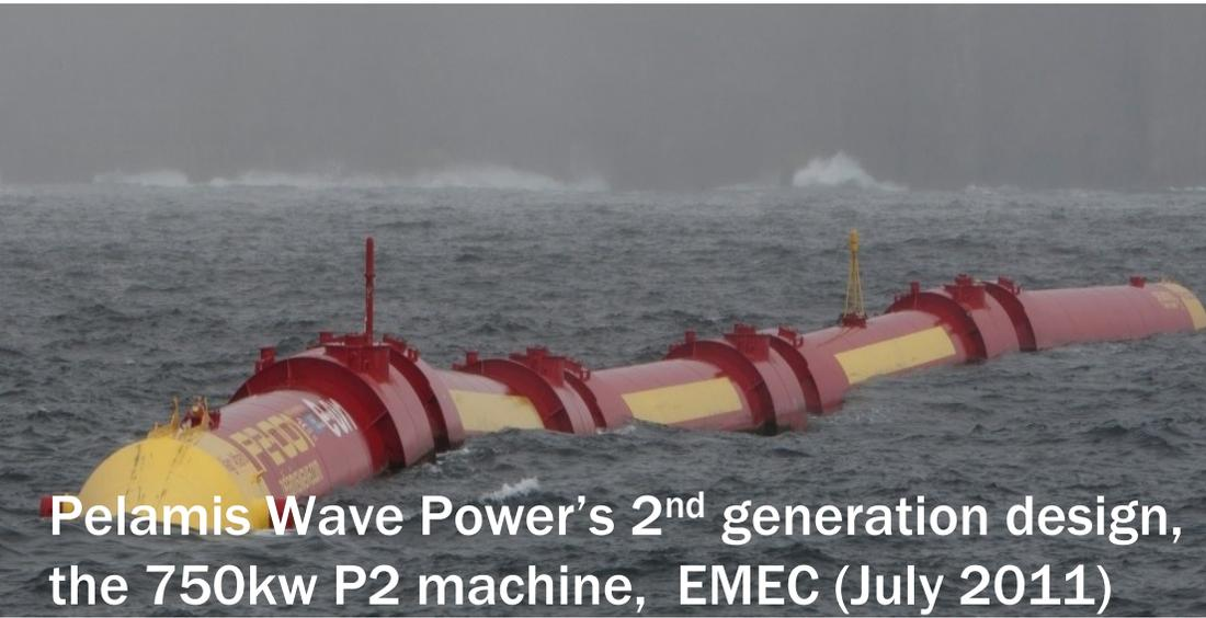
Pelamis Wave Power's 2<sup>nd</sup> generation design, the 750kw P2 machine, EMEC (July 2011)
