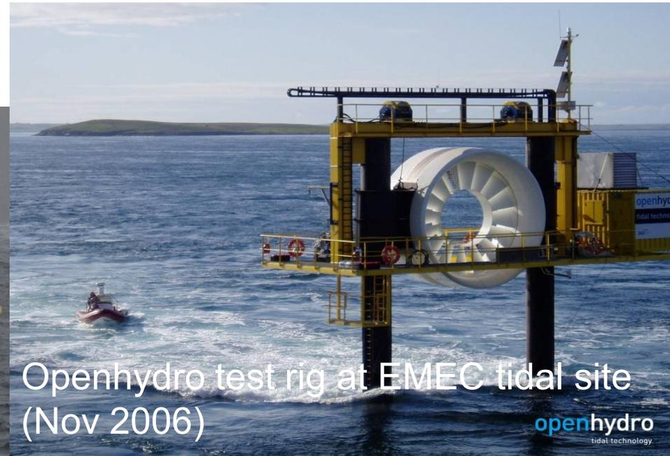
Openhydro test rig at EMEC tidal site (Nov 2006)
