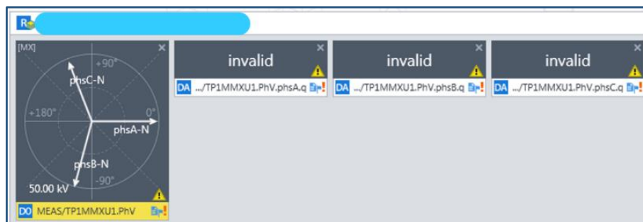
Figure 5-9. Data of Process Bus viewed in the Relays through Ied Scout
