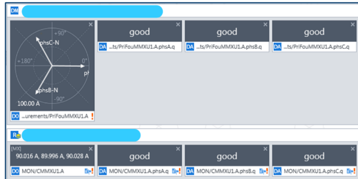
Figure 5-8. Data of Process Bus viewed in the Relays through Ied Scout
